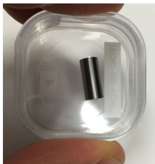
MagLIF liner machined out of S65 Be (100 ppm Fe)
